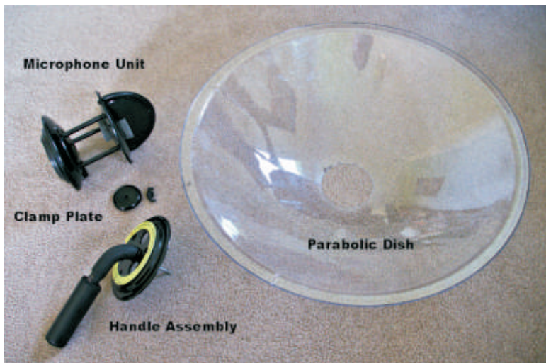
Major components of the Parabolic Microphone
